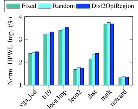
Fig. 9: Comparison between various ordering strategy in chain move on ICCAD 2014 benchmarks. “Fixed” denotes that no shuffling during each iteration of chain moves; “Random” denotes that the visiting order of cells is randomly shuffled during each iteration; “Dist2OptRegion” denotes that cells are ordered in descending order of their distances to their optimal regions during each iteration.
