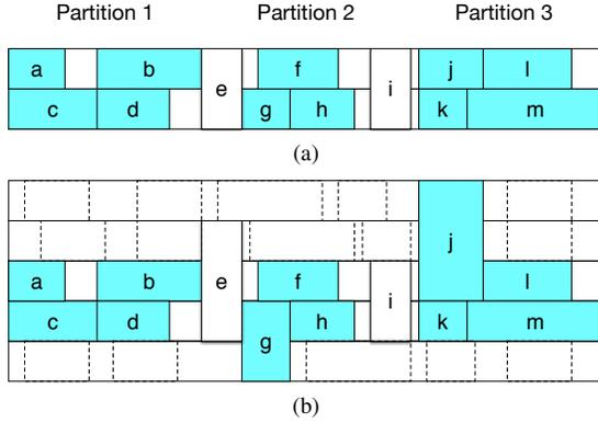
Fig. 5: Example of (a) an ideal case in ordered double-row placement (b) a general case with large splitting cells and crossing cells such as cells  $e$  and  $j$ .
