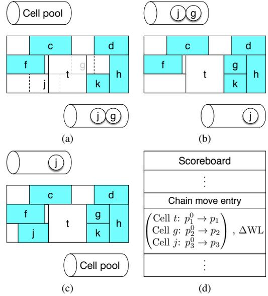
Fig. 4: A chain move example of (a) 1st movement: place cell  $t$  to  $p_1$  from  $p_1^0$  and push overlapped cell  $g$  and  $j$  to cell pool (b) 2nd movement: pop cell  $g$  from cell pool and place to  $p_2$  from  $p_2^0$  (c) 3rd movement: pop cell  $j$  from cell pool and place to  $p_3$  from  $p_3^0$  (d) corresponding chain move entry in scoreboard.
