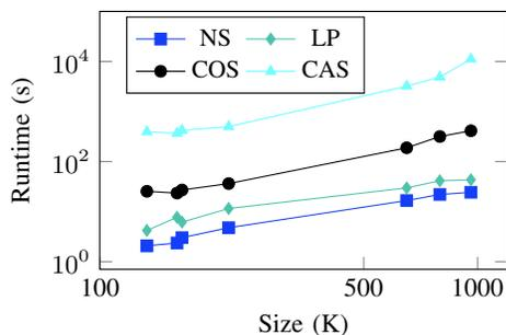
Fig. 13: Runtime comparison between various min-cost flow algorithms and linear programming to solve OMR with  $R = 18$  on various sizes of benchmarks from ICCAD 2014 benchmarks. NS: network simplex; LP: linear programming; COS: cost scaling; CAS: capacity scaling. Both axes are in log scale for easier analysis.
