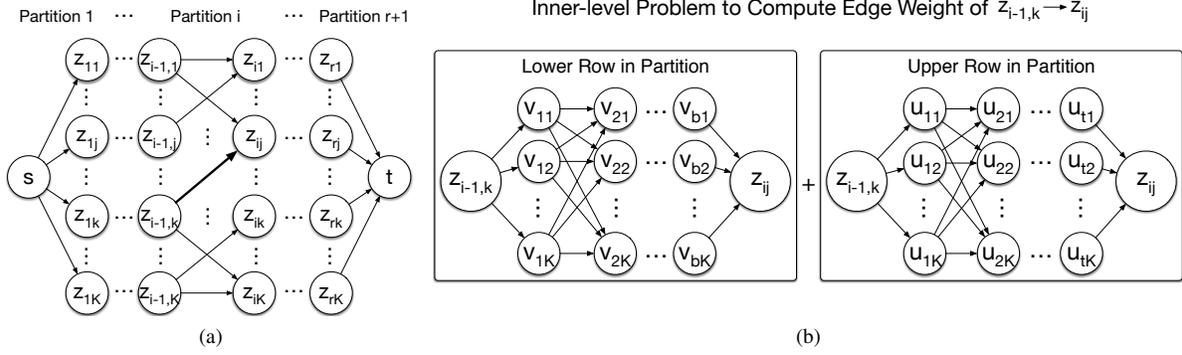
Fig. 6: (a) Outer-level shortest path problem that solves the positions of splitting cell  $z_1, z_2, \dots, z_r$ . The weights of edges in each partition need to be computed by solving the inner-level problems and (b) an inner-level problem computes the edge weight of  $z_{i-1,k} \rightarrow z_{ij}$  by solving the shortest path problem of lower and upper row in the partition with given positions of the splitting cells  $z_{i-1,k}$  and  $z_{ij}$ .
