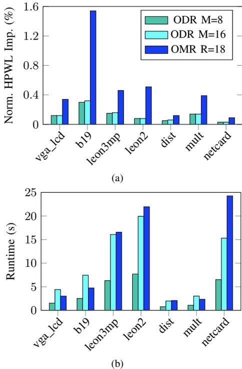
Fig. 11: Comparison between ODR (maximum displacement  $M = 8$  and  $M = 16$ ) and OMR ( $R = 18$ ) on ICCAD 2014 benchmarks. (a) HPWL improvement and (b) runtime.
