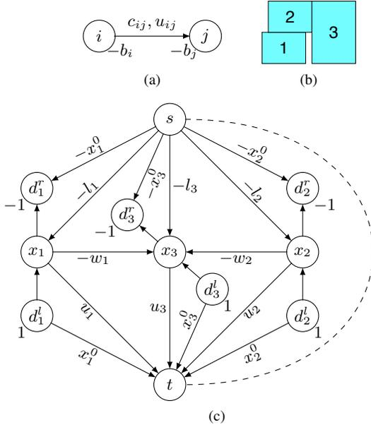
Fig. 7: (a) Mapping problem  $\mathcal{P}$  to vertices and arcs in a network flow graph where each vertex has a supply value and each arc has a cost value and a capacity value. Example of (b) three cells for ordered multiple-row placement problem  $\mathcal{P}'_m$  in Equation (11) and (c) corresponding network flow graph with non-zero vertex supply values and non-zero arc cost values labeled, while arc capacity values are not labeled.
