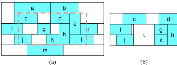
Fig. 3: Example of (a) placement with multiple-row height cells (b) inserting another cell  $t$  by slightly shifting cell  $g$  and  $j$ .
